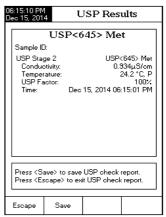
**Note:** A temperature bath at 25.0  $\pm 1$  °C is required for this measurement.
